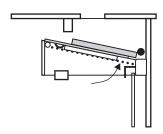
Slide the rear of the baffle on top of the rear air channel in front of the locating tabs. Make sure that the insulation is lying flat and does not obstruct the smoke from getting up the flue opening. Place hold down weights on top of the insulation - one on each side.
